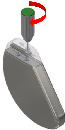
Figure 19 Tighten setscrew using the green In-line Torque Wrench
