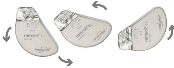
Figure 20 Proper Rotation of IPG to Wrap Excess Lead Length
