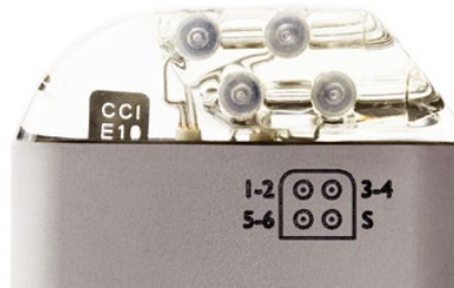
Figure 12 The remedē ® IPG Connector Block and Port Diagram
