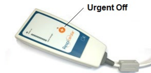
Figure 29 remedē® System Programmer Wand Urgent Off Button
