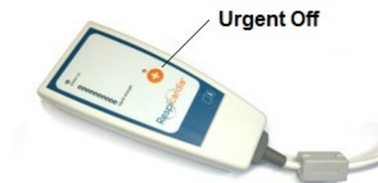
Figure 29 remedē® System Programmer Wand Urgent Off Button
